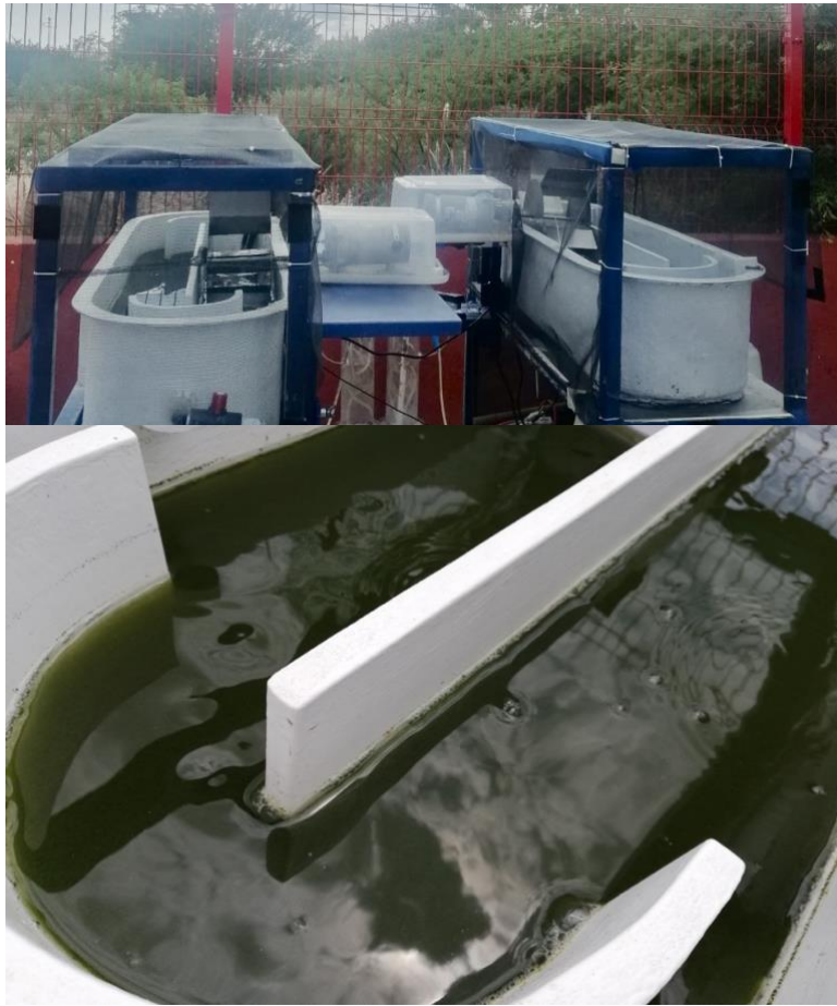
Figure S1: Outdoor HRAP systems at Querétaro, México.
