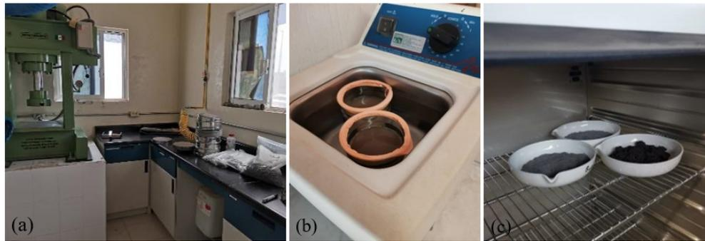
**Figure 4.5:** Pre-treatment of rock samples: (a) crushed, (b) ultrasonic washing, and drying.
