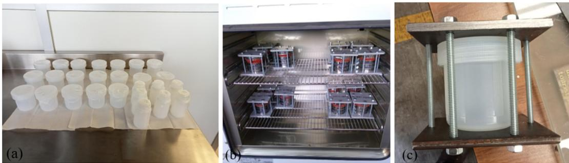
**Figure 4.7:** Experimental system: (a) teflon batch reactor, (b) Binder digital furnace, (c) metal support structure is employed to prevent steam leakage resulting from high temperature.
