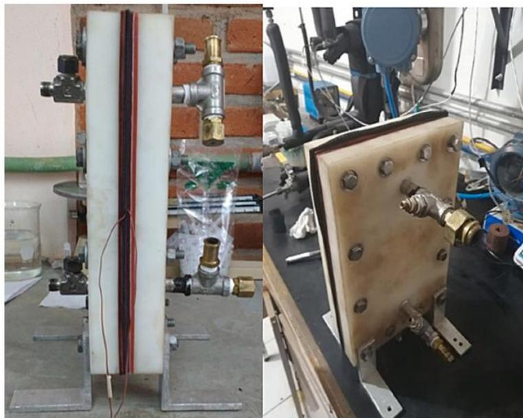
Fig. 6. Hydrophobic porous membrane desorber/condenser experimental module.
