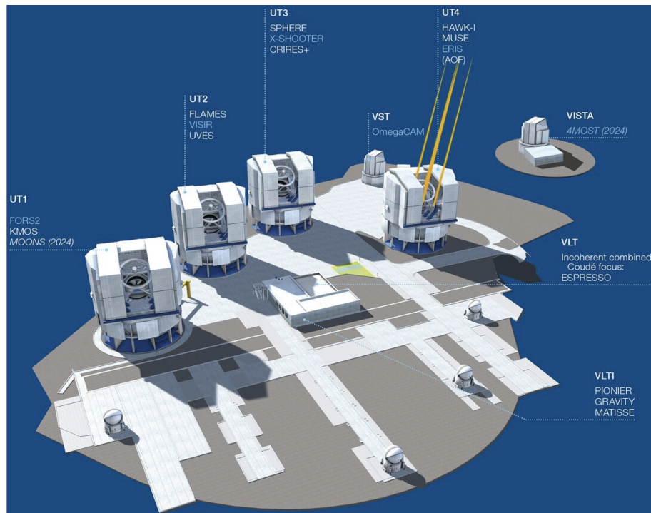
Figure 2.9: The Paranal Observatory telescopes. The instruments listed in italics are not yet in operation. The year in brackets indicates the start of operations. Image taken from the ESO webpage .
