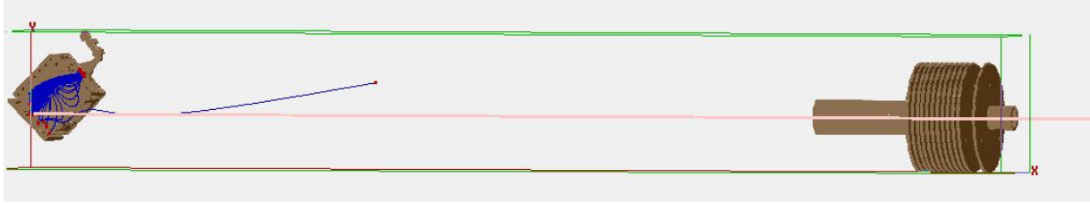
Figure 4.4: Simulation of neutral atoms (shown in pink) emerging from right to left from the interaction region, through the Field Ionizer and up to the NPD. The impacts of the ions are depicted in red and the secondary emitted electrons are displayed in blue.
