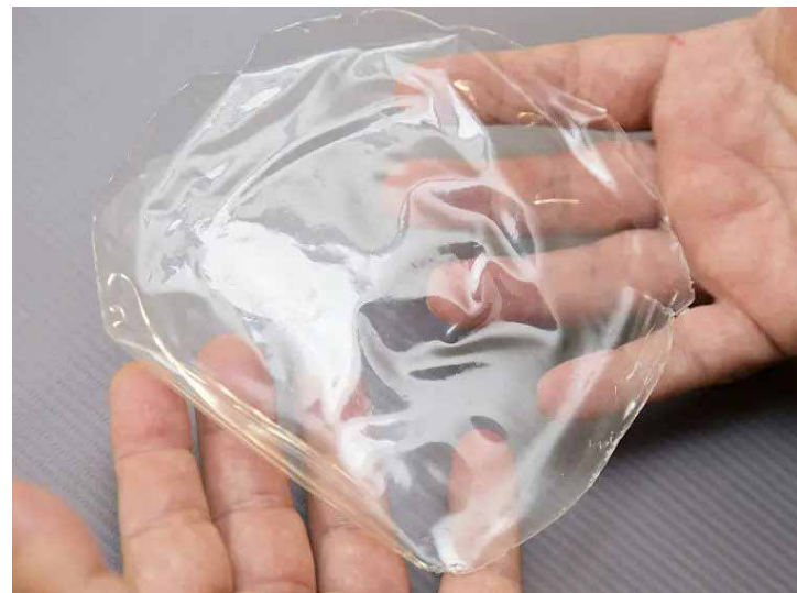
Figura 11. Film plástico realizado a partir de almidones de yuca. Gerhard Waller, SciDevNet, 2019, ( https://www.scidev.net/america-latina/news/fabrican-plastico-biodegradable-con-almidon-de-yuca )
