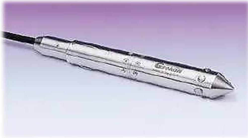
Imagen 21: Celda USBM Borehole Deformation Gauge. Fuente: (Blondel Buijuy, 2017)
