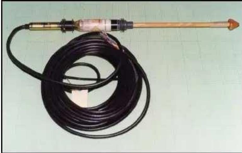
Imagen 24: Celda Hollow Inclusion. Fuente: : (Blondel Buijuy, 2017)
