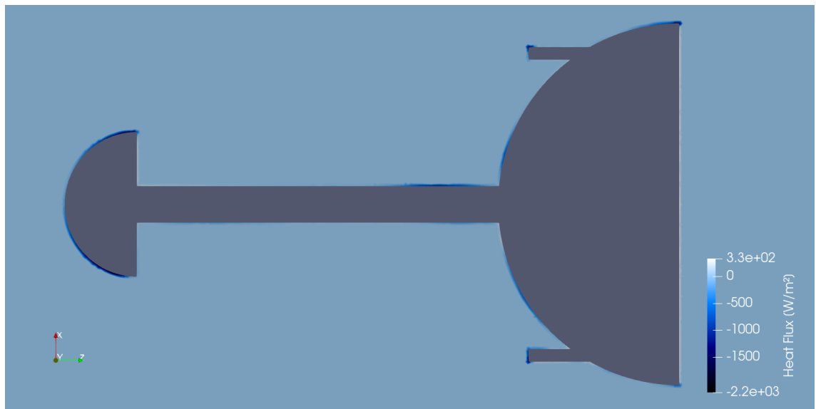
Figure 68: Surface Fluid Heat Flux of Ringed Body 1 at Mach 2 and 16° AoA.
