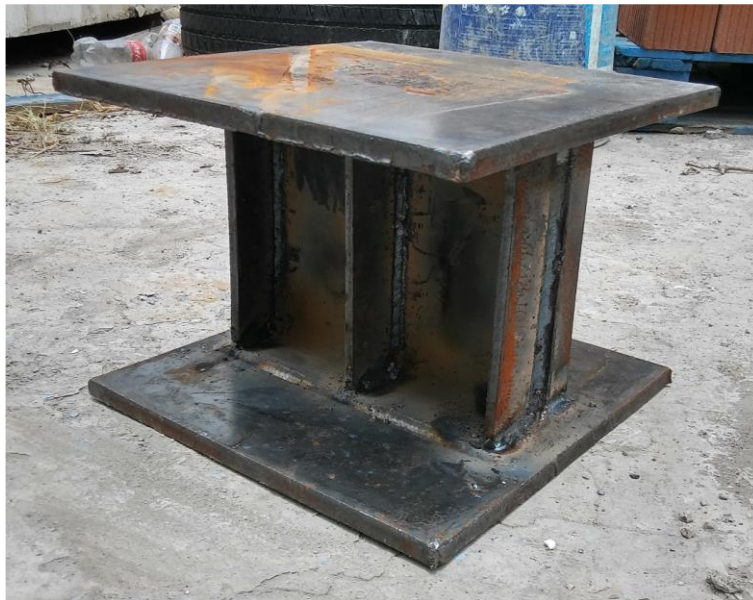
Figure 5-5. I-damper of specimen P-ID-1.
