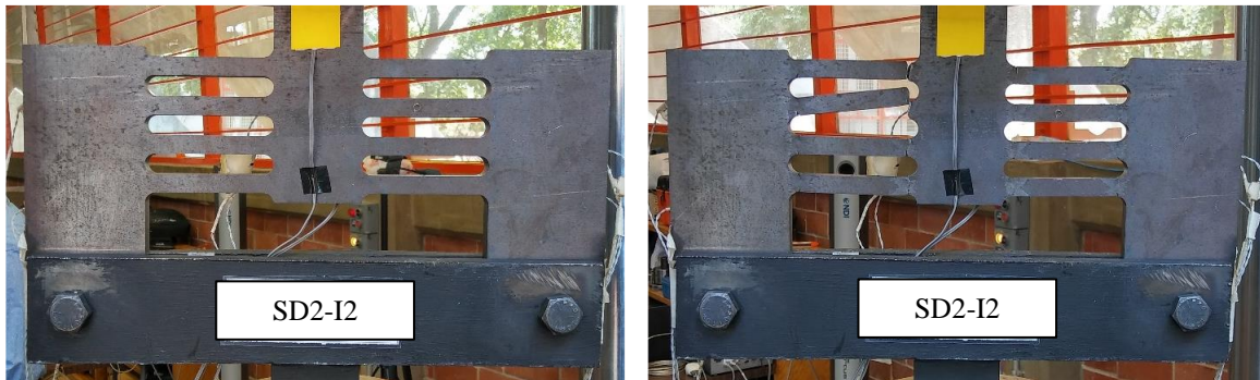
Figure 7-17. Specimen SD2-I2 before and after testing.
