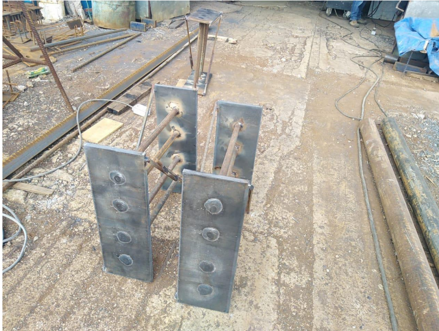
Figure 6-47. Dumbbell connection assembly.
