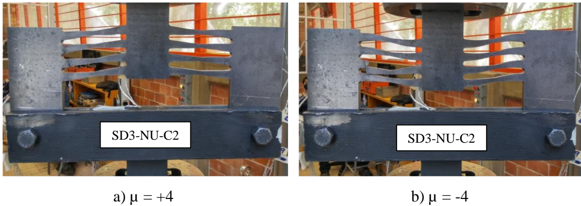
Figure 7-25. Failure modes of SD3-NU-C2.
