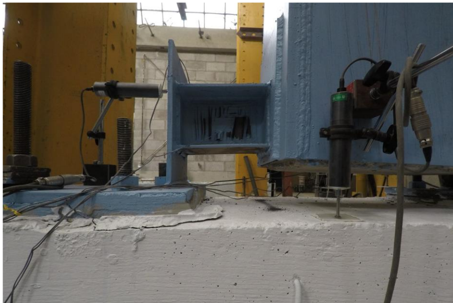
Figure 5-25. Damper deformation at -0.025 drift (specimen P-ID-2).
