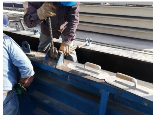
b) Formwork securing
