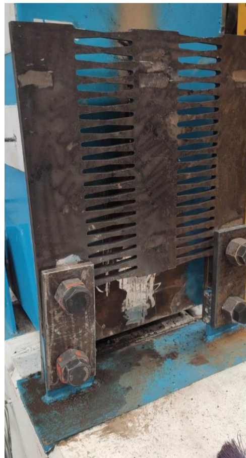
Figure 6-38. Bolted configuration for specimen P-SD-2R.
