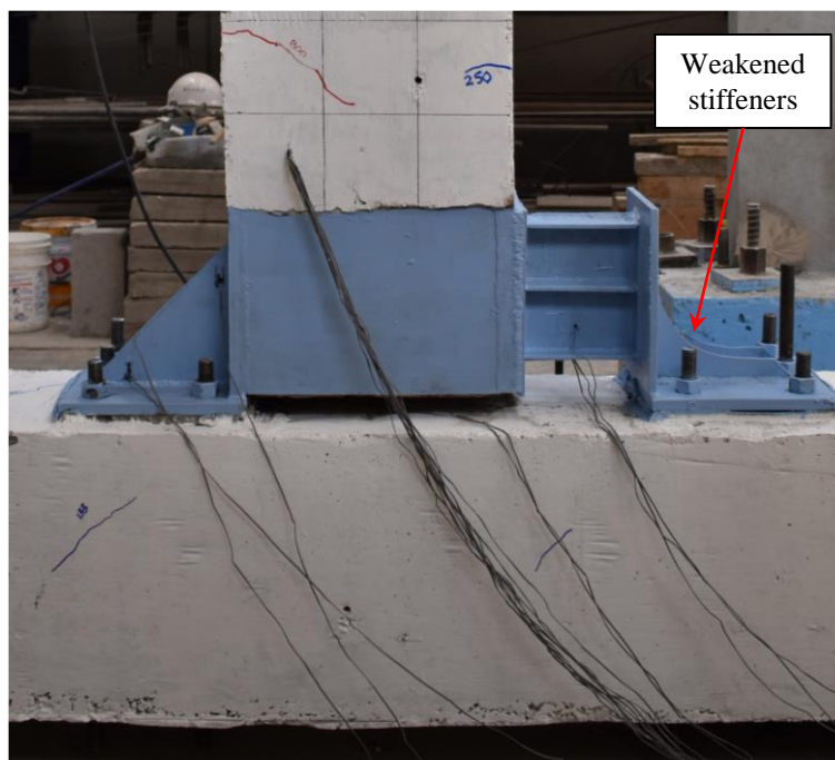
Figure 5-8. Connection of specimen P-ID-1M with weakened stiffeners.
