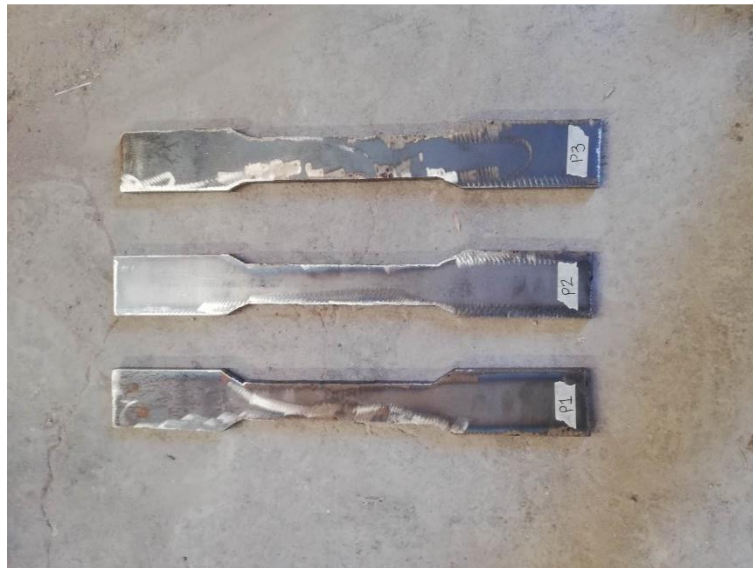
Figure 6-41. Structural steel coupons.
