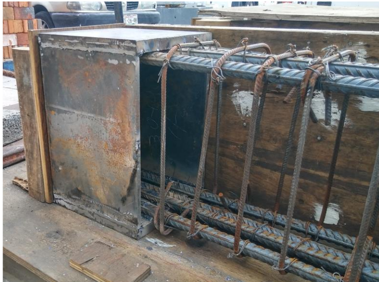
Figure 5-2. Steel box and welded longitudinal reinforcement of the beam.
