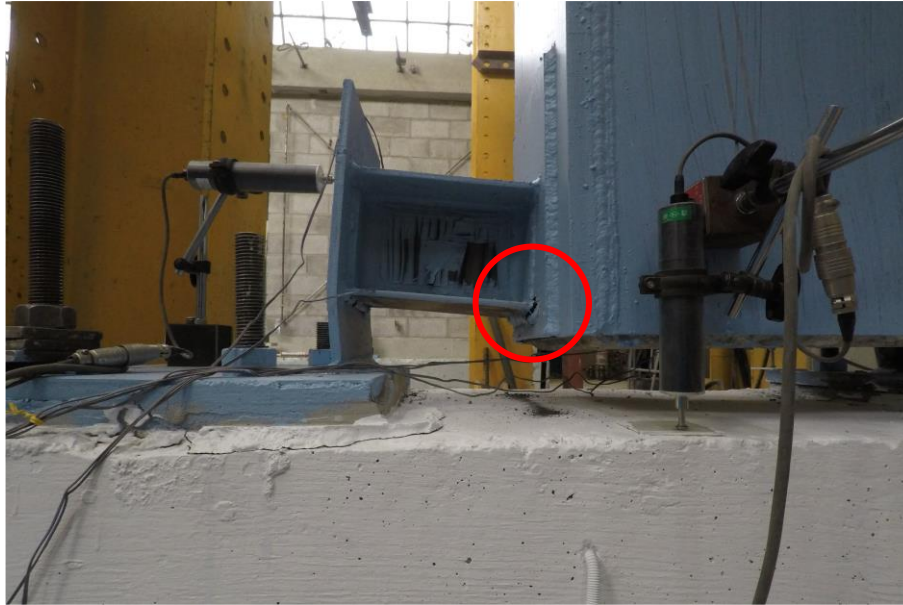
Figure 5-24. Damper deformation at 0.025 drift (specimen P-ID-2).
