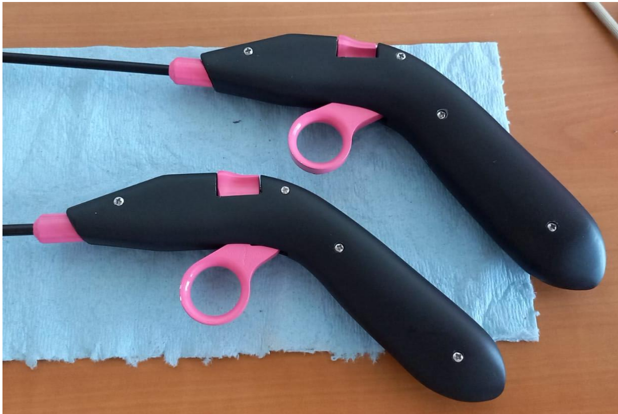
Figura 51 Prototipos N5, pinza grasper y maryland.
