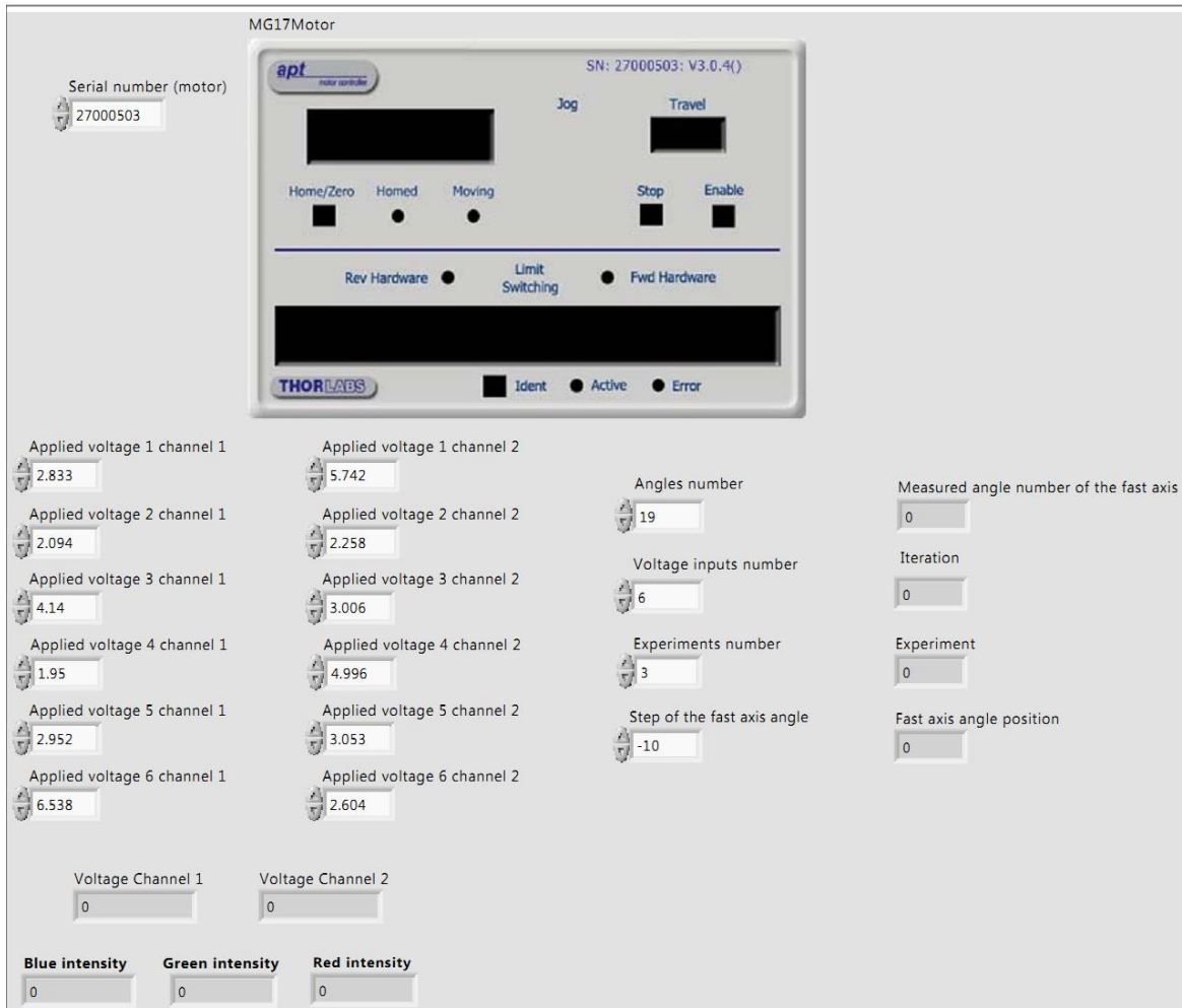
Figure C1: front panel of the LabView program to control the Stokes polarimeter. The inputs are the number of voltages to set up for each channel, the configuration voltage values to apply, also, the angle and experiment numbers to analyze, and finally, the step to rotate the principal axis of the sample. In the output, the front panel shows the voltage applied to the current iteration, the angle and experiment numbers, the current position of the principal axis angle, and finally, the current intensity value measured for each wavelength.
