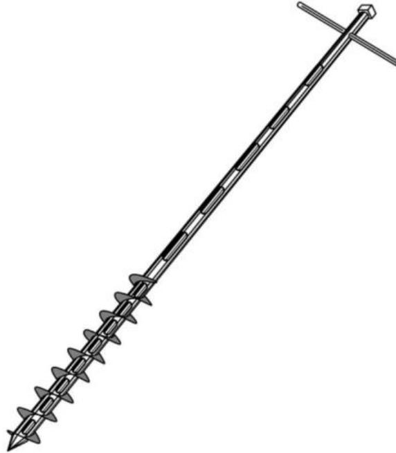
**Figura 10.** Muestreador de ranura de 2 niveles con punta de barrena. ASTM international (2015) [imagen], “Standard Practices for Sampling Metal Powders” (p.3).
