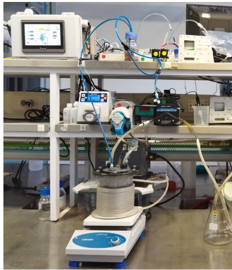
Fig. 6. Hydrogen producing reactor.
