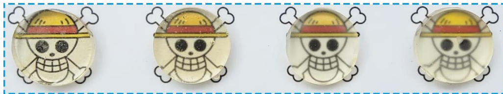
Figure 39. The reduction in transmittance is visually appreciable. (From left to right: 0, 0.3 0.5 and 1.0 wt% S-CNC.)
