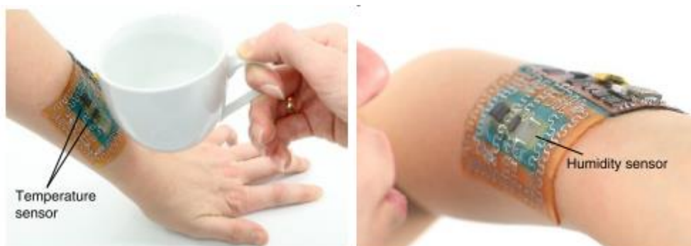
Figure 9. Double stimuli response sensor based on a gelatin hydrogel and other biocompatible elements. Nat. Matter. 19, 1102-1109 (2020).
