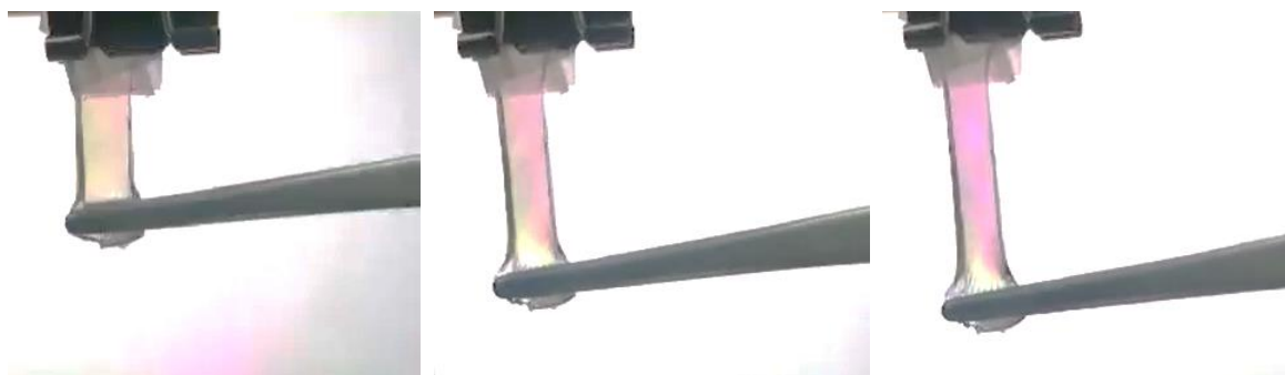
Figure 42. Shear-birefringence effect shown by the 1.0 wt% S-CNC eutectogel under polarized light (Samsung Galaxy Tab S7). The effect intensifies as the material is stretched.
