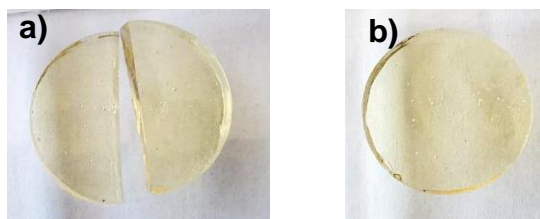
Figure 51. Self-healing displayed by the eutectogels. a) Sample before being heated up to 50\text{ }^{\circ}\text{C} . b) Gel after being casted and cooled again at 4\text{ }^{\circ}\text{C} overnight.
