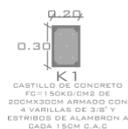
CABILLO DE CONCRETO  $f'c = 150\text{KG/CM}^2$  DE  $20\text{CM} \times 30\text{CM}$  ARMADO CON 4 VARILLAS DE  $3/8"$  Y ESTRIBOS DE ALAMBRE A CADA  $15\text{CM}$  C.A.C
