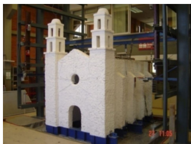
Figure 2.25. Experimental model of a typical colonial church of Puebla, Mexico (Chávez, 2010)
