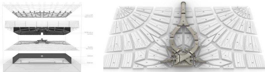
Fig. 18. 3D-Printed Formwork for Integrated Funicular Concrete Slabs.
