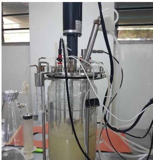
Figura 32. Biorreactor BioFlo<sup>®</sup>/CelliGen<sup>®</sup> 115, New Brunswick.
