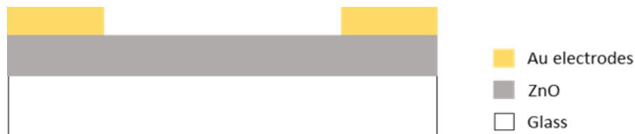
Figure 4.13. Device I schematic representation. The difference between Structure Ia and Ib lies in the concentration of the ZnO deposited layer.
