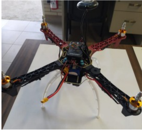
Figure 7.12: quadrotor developed in our laboratory
