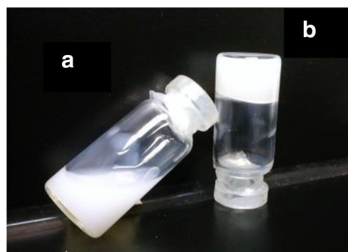
Fig. 4 Tubes showing the behavior of the PF127:PF68 gel (proportion 8:2) with nanoparticles, at different temperatures. (a) At 27 °C (low viscosity). (b) At 37 °C (gel formed)
