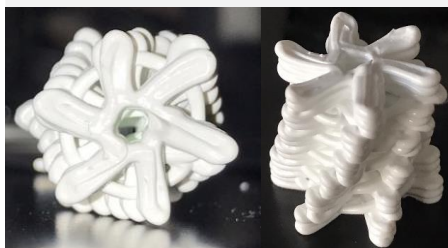
3D hexahelicoidal hierarchical structures of entirely TiO 2 composition
