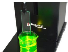
Figura 1. 9. Dip coating (Innovations, 2012)
