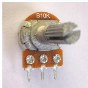
**Fig 2.2c** Potenciómetro (2021). Licencia libre de uso: [https://commons.wikimedia.org/wiki/File:10K\\_Potentiometer\\_1480310\\_1\\_2\\_Enhancer.jpg](https://commons.wikimedia.org/wiki/File:10K_Potentiometer_1480310_1_2_Enhancer.jpg)
