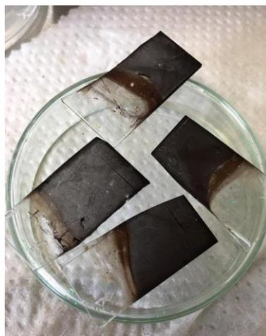
**FIGURA 20: PELÍCULAS DELGADAS DE  $\text{CuO}$  DESPUÉS DEL TRATAMIENTO TÉRMICO.**
