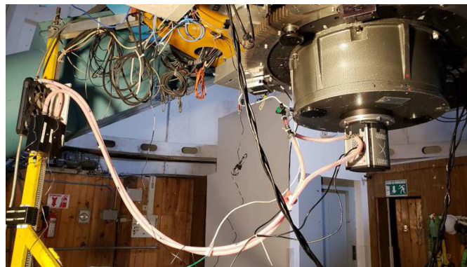
Fig. 3 In this picture we show the physical distribution of the system. To the right, the camera is attached to the telescope and the hoses run to the pump and the radiator which are also attached to the telescope. Once installed, the hose is filled using the green faucet.
