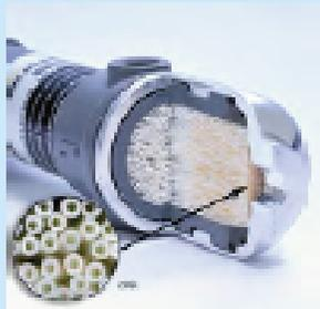
A typical membrane separator contains thousands of fibers, which are bundled and encased at both ends in epoxy resin. The ends of the bundles are cut, which leaves the fiber bores open on both ends, allowing the gas to travel from one end to the other. The bundles of fibers are enclosed in a suitable casing which protects the fibers and routes the gas properly.
