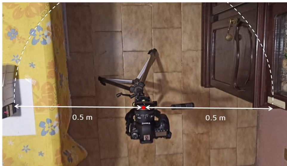
Figure 3.12: Aerial view of the camera set up to determine real angle of view of the lens.
