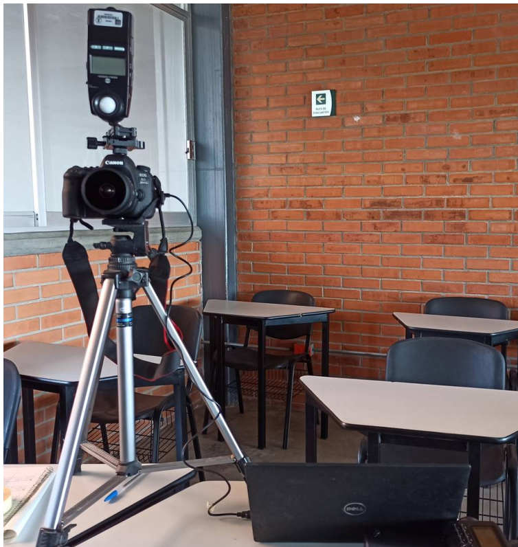
Figure 3.16: Illuminance meter positioned above the fisheye lens.
