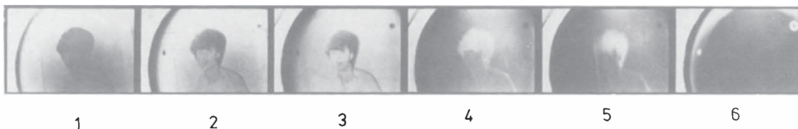
Fig. 1 Light-sensitive BZ reaction (composition 1; Table 1) with a negative image projected onto it. Frame 1: appearance of an image; 2, 3: positive image; 4, 5: negative image; 6: transient phase. The cycle shown here then recurs.
