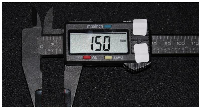
Figura 8 Calibrador digital, SATA 9151, 0-150MM.
