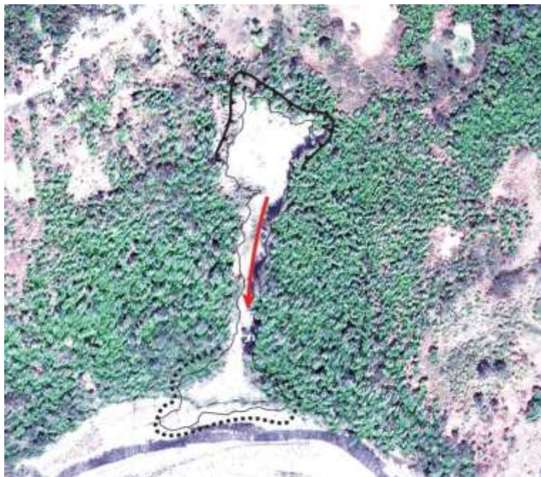
Figure 35. A debris flow in a 3D view based on a very high-resolution digital elevation model derived from GeoEye-1 stereo-pairs. The source area, channel, and deposit area (partially removed by the river) are visible.
