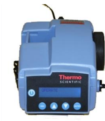
Figura 6.3. Monitor de aerosoles personal pDR-1500 Thermo Scientific (Thermo Scientific, 2008).
