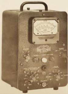
**USES:** The D-C Amplifier and Electrometer is basically a millivoltmeter with extremely high input resistance. It measures:
