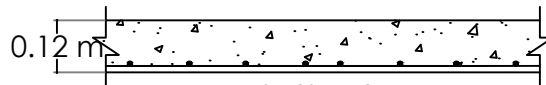
DETALLE 9.- LOSA MACIZA h = 12 cm V's 3 @ 20 cm AMBOS SENTIDOS CONCRETO F'C=200 KG/CM 2
