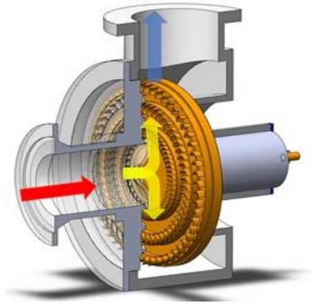
Fig. 22 " Turbina de salida radial (Spadacini, et al., 2015) "
