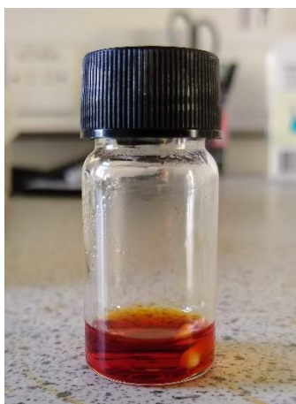
Figure 8. LaFeO 3 polymeric template solution to prepare the spin-coated films.
