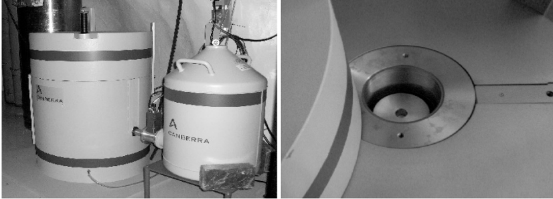
Figure 2.10: Canberra HPGe well-type detector: (a) Shielding and Nitrogen dewar horizontally arranged. (b) Detector sample chamber [22]
