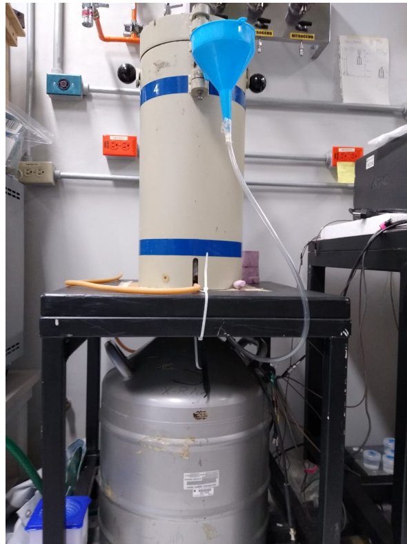
Figure 3.2: Experimental setup of ICN-UNAM HPGe detector: (a) Upper view of the cryostat head and the shells of the whole shielding. (b) Front view of the detector with shielding and Nitrogen Dewar installed.
