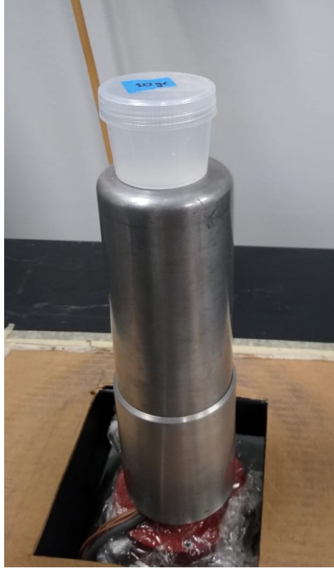
Figure 3.13: Extended sample of diluted salt substitute in injectable solution into a polypropylene container placed at the top of the ICN HPGe detector's head.
