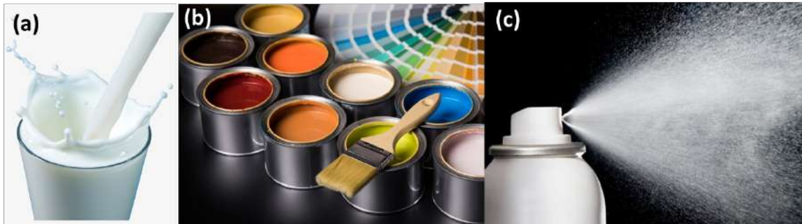
Figure 3.1: Examples of colloidal systems present in everyday life. (a) Milk is a colloidal suspension named emulsion: liquid fat-globules are suspended in water. (b) Paint is a colloidal system named sol, where solid pigment particles are suspended in a liquid solvent solution. (c) Sprays in cosmetics are colloidal systems called aerosol consisting of liquid particles suspended in air or other gas.
