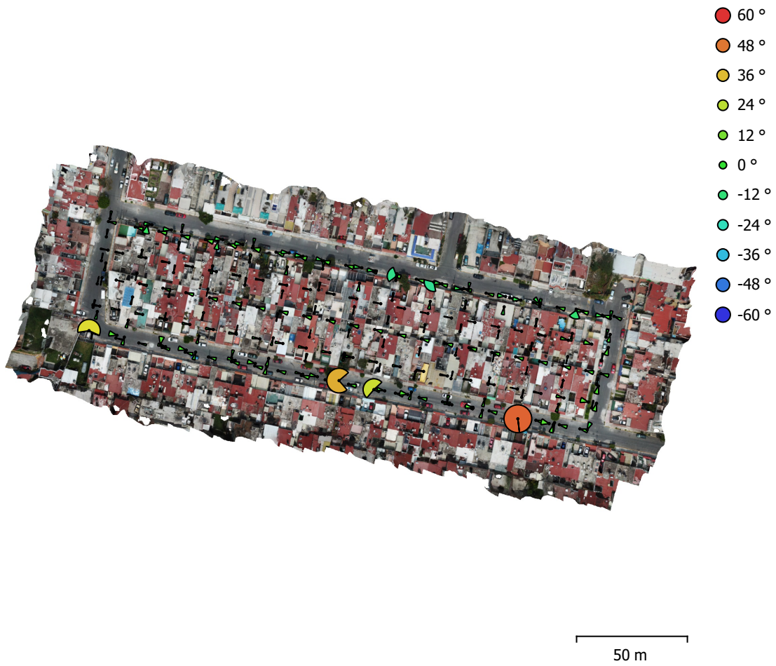
Fig. 4. Camera orientations and error estimates. Arcs represent yaw error estimates.
