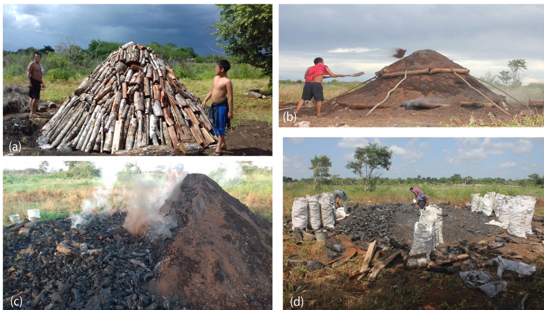
Fig. 3 The main stages of artisanal charcoal production with earth kilns. The firewood is piled in the form of a volcano (a), then the volcano is covered with dry grass and soil. While it burns, the oven is regularly visited (two or three times daily) to verify that the charcoal transformation process is proceeding adequately (b). When this
