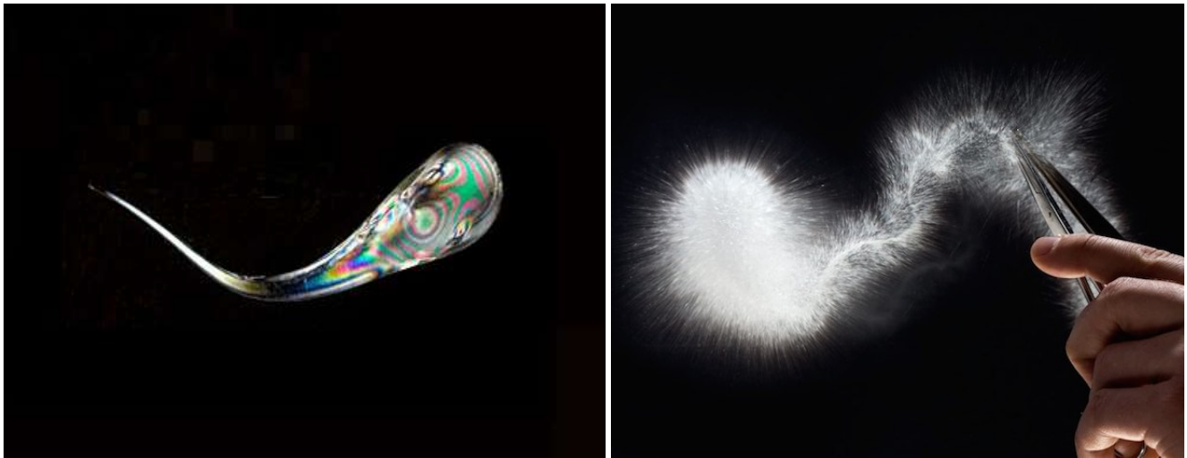
Figure 1.2: left) Prince Rupert's drop. The color fringes is indicative of residual stresses. right) Prince Rupert's drop right after the tail of the drop is cut off. The drop shatters to pieces given the internal stresses this glass has, given the preparation protocol. This also gives PRDs exceptional strength properties (see main text for further details). Taken from the web.
