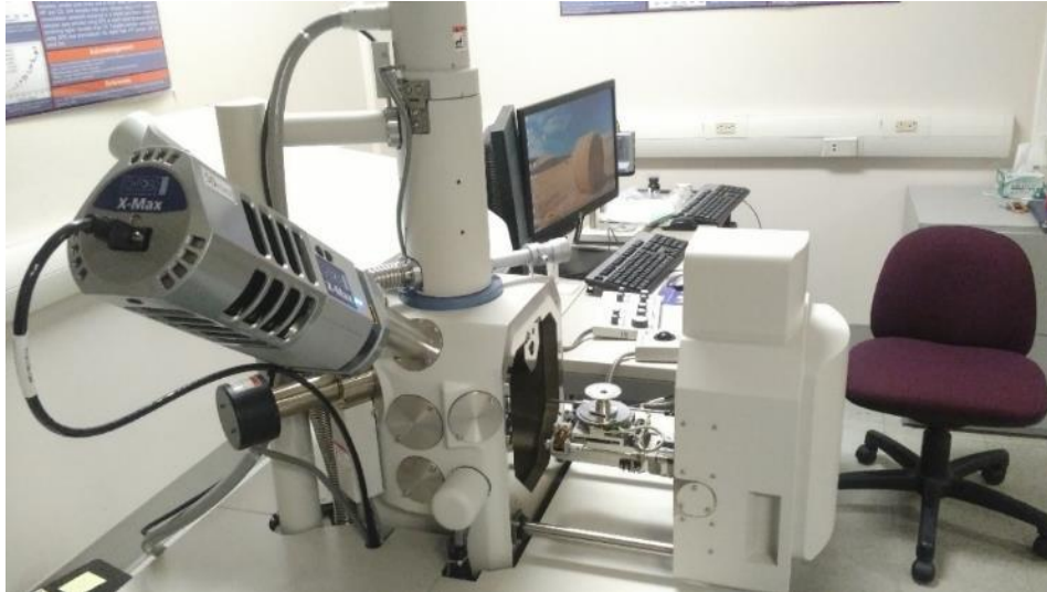
Fig 3.1. Hitachi-3400-N-II Analytical Scanning Electron Microscope, SEM (Boise State University).
