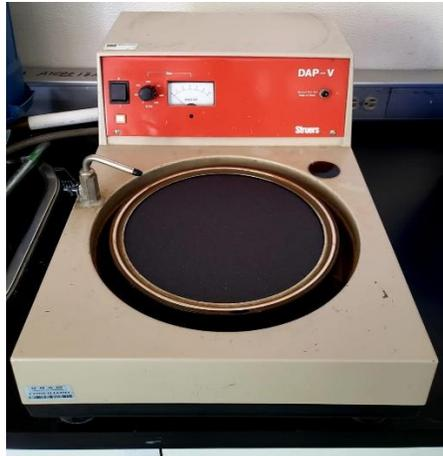
**Figura 4.12.** Maquina pulidora Struers.
