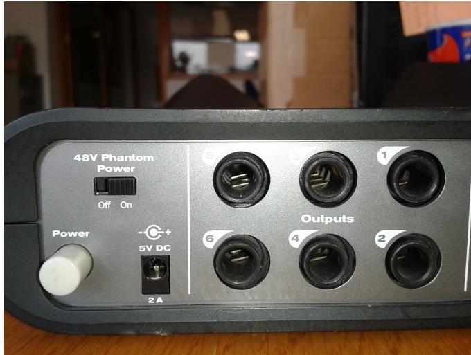
Figura 3.1: Interruptor del Phantom Power .
