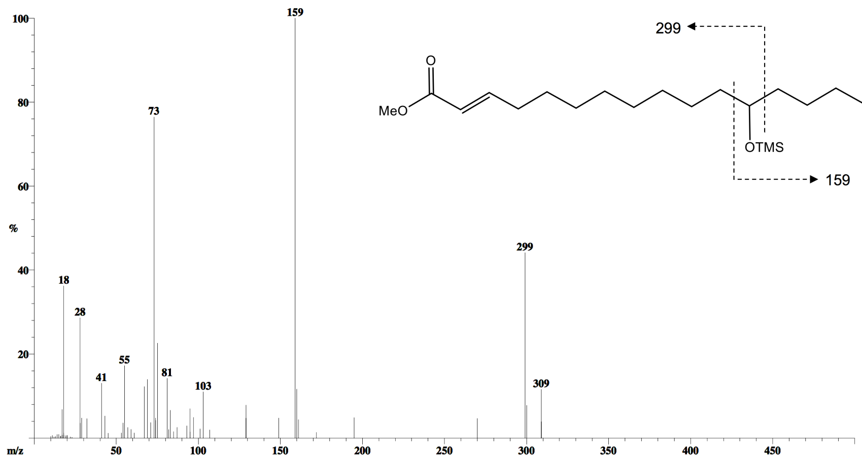
Figure S79. EIMS of silylated 12-hydroxy-2-hexadecenoic acid methyl ester: m/z 299 ( [C_{13}H_{22}O_3TMS]^+ ) and 159 ( [C_5H_{10}OTMS]^+ ).
