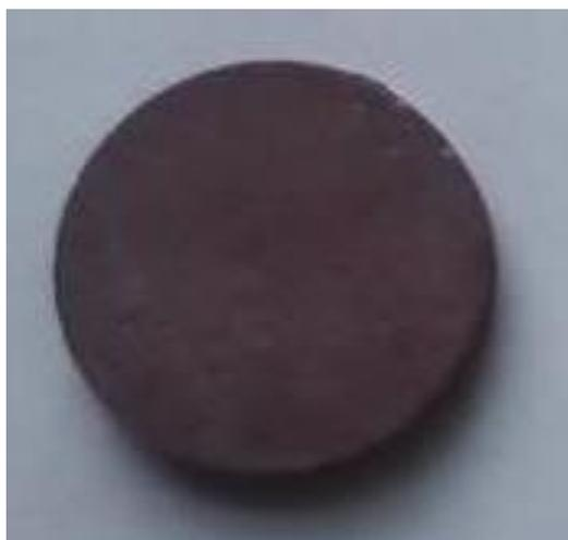
Figura 15. Pastilla 98.49% Cu-1.40%Dy<sub>2</sub>O<sub>3</sub>
