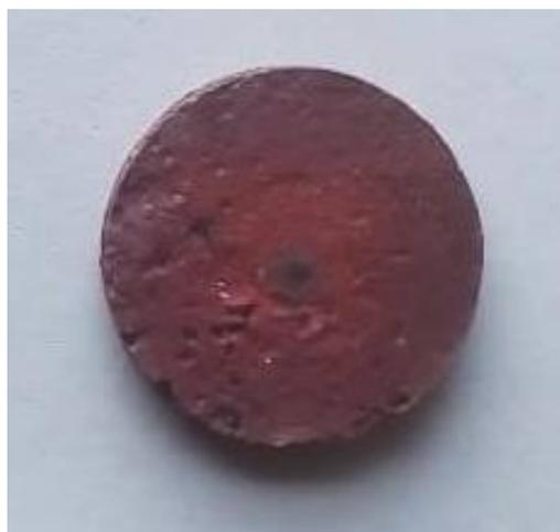
Figura 16. Pastilla 98.49% Cu-1.40%Pr<sub>6</sub>O<sub>11</sub>
