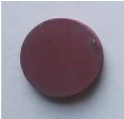
Figura 14. Pastilla 98.49% Cu-1.40%Sm<sub>2</sub>O<sub>3</sub>
