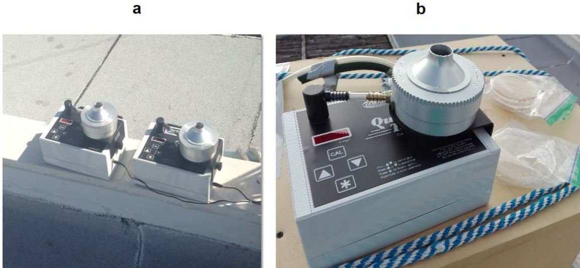
Figura 2.7. QuickTake30 Sample Pump Standard Biostage. (a) Muestreo invierno-2017, (b) verano- 2018.
