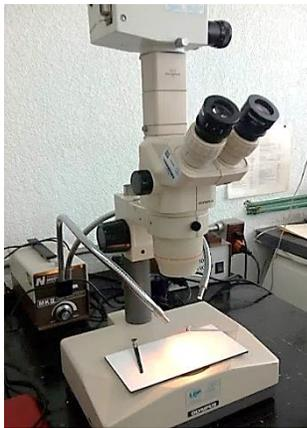
*Figura 3.6: Estereoscopio Olympus ST-PT.*
