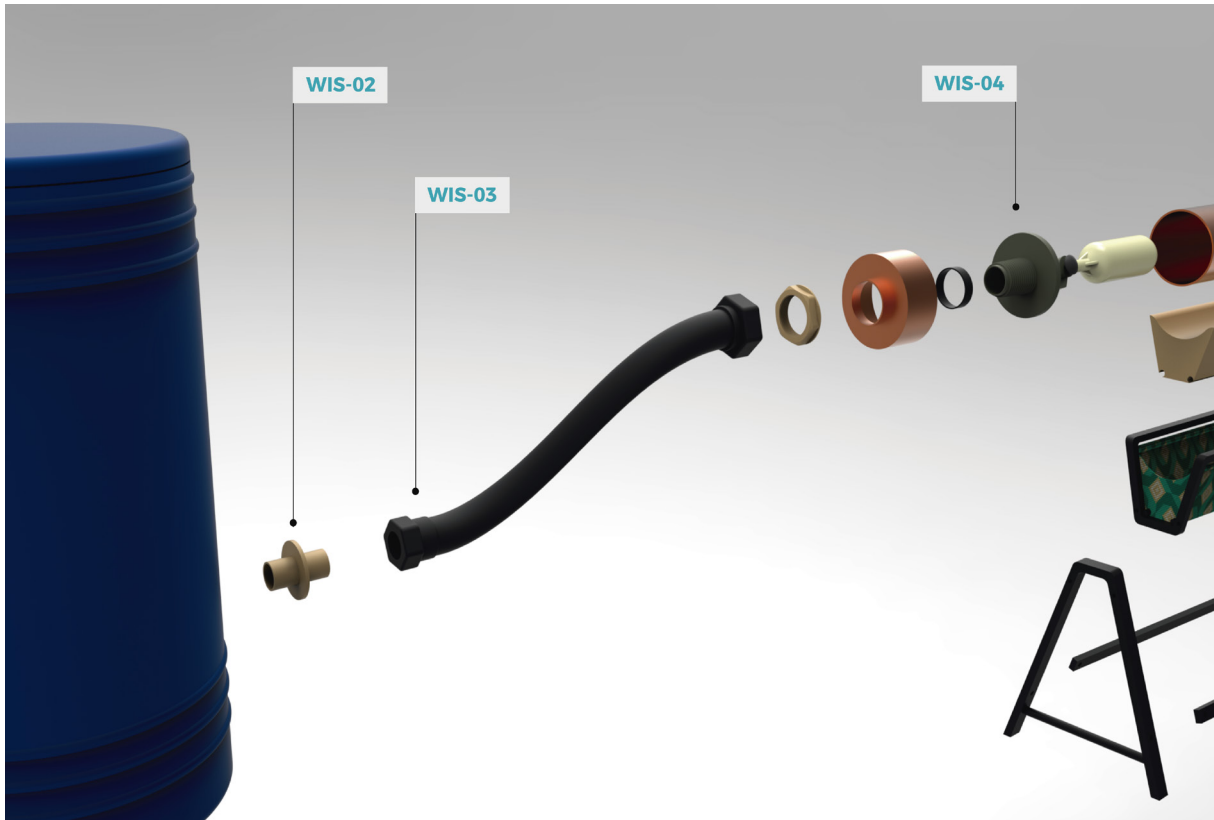
Figure 35. Water Input System, exploited View
