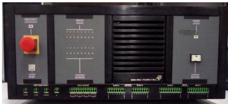
Figura 22: Controlador Eshed Robotec Controller-B ACL
